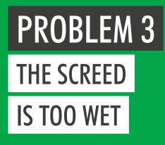
A high moisture content can cause the screed to give off a damp aroma and will seriously impair the quality of the finish.
